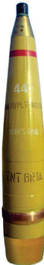
It is a high explosive extended range (HEER) Shell. Better fragmentation is achieved by introducing high quality steel alloy and thinning the body of the shell. The optimised ballistic shape of the shell improve the ballistic coefficient (Reduced drag) & provide better accuracy. The Base Bleed Unit (BBU) at base reduces the drag and gives additional thrust to carry the shell further.
