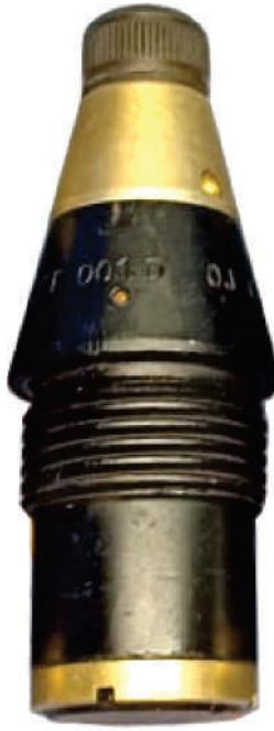
Fuze B429 is a percussion type of nose fuze having direct, delay and Graze action. This fuze is used for Shell 130 mm HE Filled. The fuze can be set externally to 'I' and 'D' mode corresponding to '0' and '3' markings on fuze body respectively with the help of selector mechanism incorporated in fuze body.
